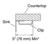
\* Allow clearance around sink rim for clip attachment.
